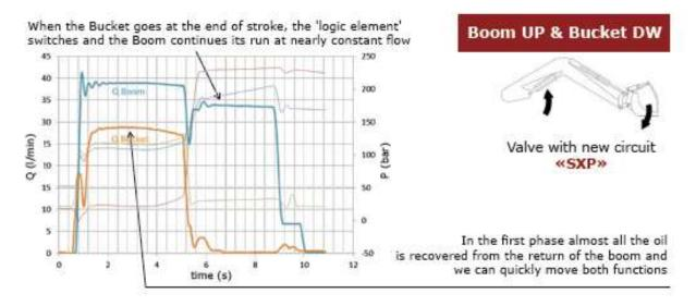
Above all, the increase in productivity of the front loader makes Walvoil SXP's innovation worthwhile. Thanks to the skillful use of the Series circuit, that makes the most out of the pump flow, bench tests and functional field tests in collaboration with international OEMs have shown a reduction up to 20% of the loading and unloading cycle times compared to a traditional parallel circuit.
