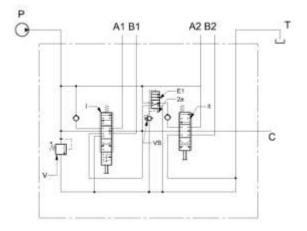
When the pressure on the P channel reaches the calibration value of the VS valve (for example when a function is reaching its stroke end), the logic element switches to the second working position, connecting S channel to tank and the simultaneous opening of the P parallel channel.
