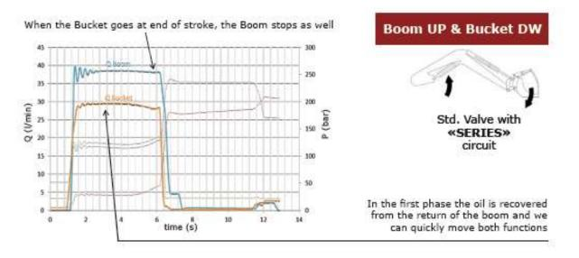
In traditional Series circuits, during the simultaneous operation of two functions (typically arm lifting and bucket movement), if the cylinders of a function reach their stroke end, also the cylinders of the other function stop, creating an obvious discomfort to the operator. This is one of the main problems afflicting these circuits, in addition to the pressure summation of the two functions, which limits the maximum load capacity. (*pic. #5*).
